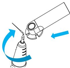
When you set the tip on the device, the tip can be set within a range of 10°, therefore, do not tighten the tip in excess.
